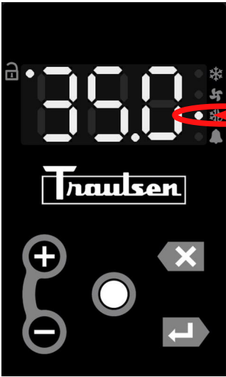
Fig. 4.4a Defrost Icon Illuminates In Electric Defrost ONLY
