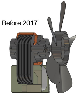
Fig. 6B.12.1e SHADED POLE MOTOR (PRE 2017) R450 TRAULSEN P/N 338-60054-00
